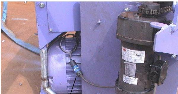
Swing the magnet around and disconnect the magnet drive power cord.
