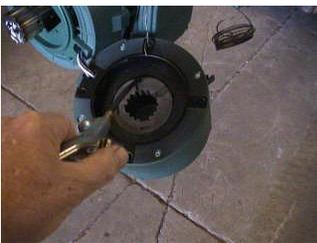
7. After the disc is cleaned, slide the assembly back onto the motor shaft and install the bolts.
