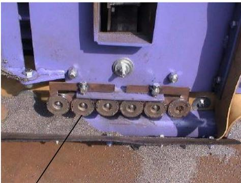
Slide the magnet mount in place as shown. Secure with lock down bolts.
