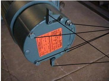
5. Slip the brake assembly off of the motor shaft being careful not to pull on the brake electrical wires. Use bailing wire to support the brake so no stress will be put on the wires while you clean the brake.
