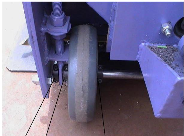
With the unit still lifted slightly off the floor, remove the (3) split collars that hold the front tires in place. Remove the axle and tires.
