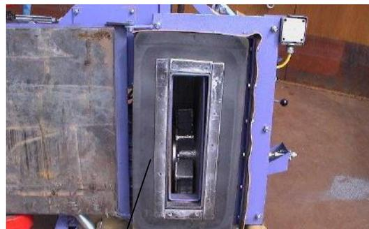
Place the seal on the wall blast plate as shown.
