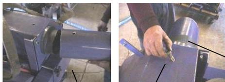
**Step 13** Install the exhaust tube and locking pin. Caution- make sure that the rubber seal is in place and properly attached.
