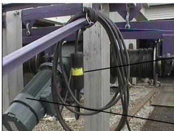
Connect the power cable from the Drive Wheel Assembly to the power supply cable from the hoist. The power supply is 15' long- the extra length is required when used on the floating roof fixture. Roll up the excess cable and tie secure it to the fixture frame.
