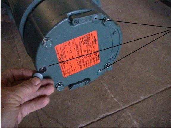
Remove the three plugs on the end of the brake. Tighten each of the three Allen head bolt  $\frac{1}{4}$  turn and try the hoist again. Continue this procedure until the brake works properly.
