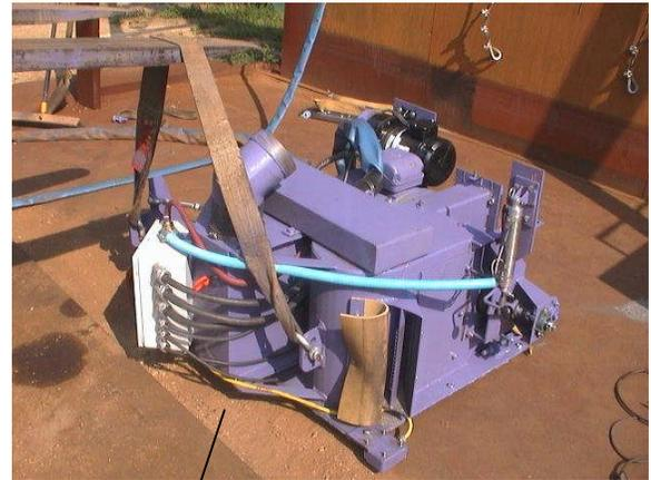
Using a fork lift, strap and shackles, lower the machine on its back side as shown.
