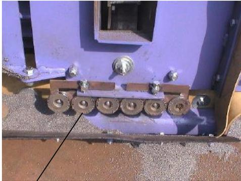
Remove the magnet mount by loosening
