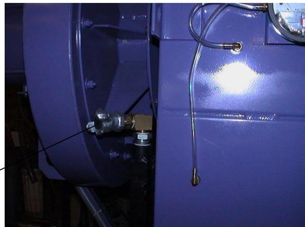
Connect a 3/4" air line with a Chicago fitting to the dust collector air fitting. The pulsing system will automatically keep the cartridge filters clean. A smaller air line can be adapted if required.
