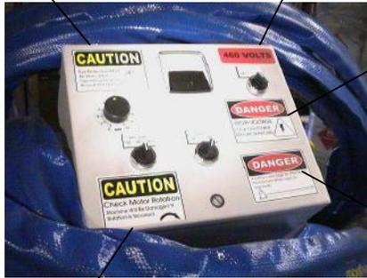
A safety cable must be attached to this machine when used on tank roofs.
