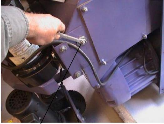
Loosen the nut holding the side bracket
