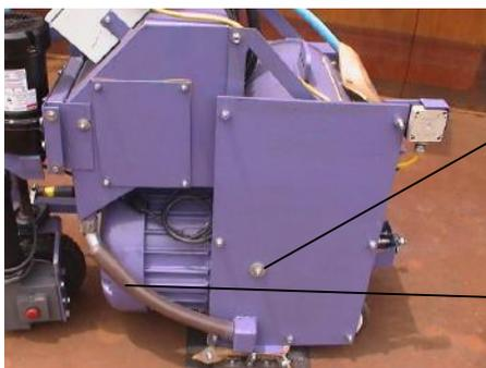
Set the side cover plate in place over the liner stud. Install
