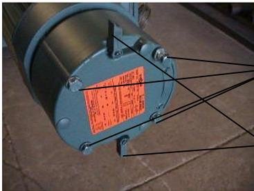
4. Open the brake release arms ( this spreads the brake spring plates and allows the disc to turn freely.
