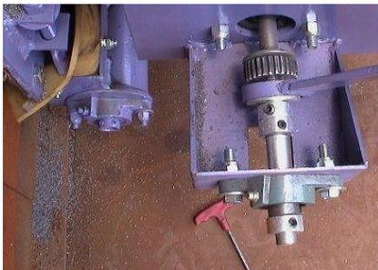
Slide the control cage arm off of the cog hub by loosening the retaining collar and rocking the arm back and forth until it comes off.
