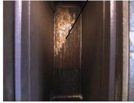
There are two liners in the machine that are used in the machine for both horizontal and vertical operation- the Top curved liner and the back wall liner. Inspect these liners for wear at 50 hour intervals. If wear is found, remove the liners and fill the wear area with hard face weld. If the wear is too great, replace the liner.
