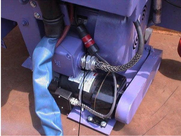
Plug in the screw drive motor. Make sure the Red coded plug is connected to the red coded Receptacle.
