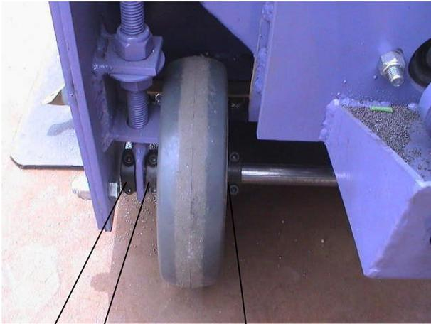
Slide the left tire onto the axle and the axle into the right adjustable support. Make sure the (3) split collars are positioned on each side of the tire and at the end of the axle shaft as shown above. Tighten all collars.
