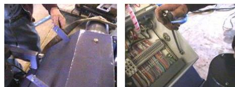
**Step 14** Attach the control panel to the hopper Tabs as shown.
