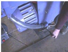
**Step 15** Reinstall the hopper drain hose.
