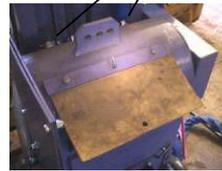
Remove nuts and washers to remove the top curved liner.
