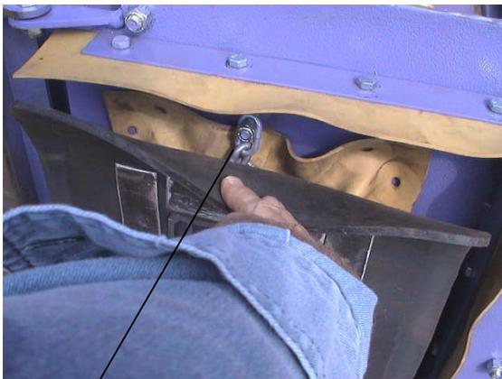
Remove the lock nut holding the seal Chain support from both the top and Bottom of the seal assembly.
