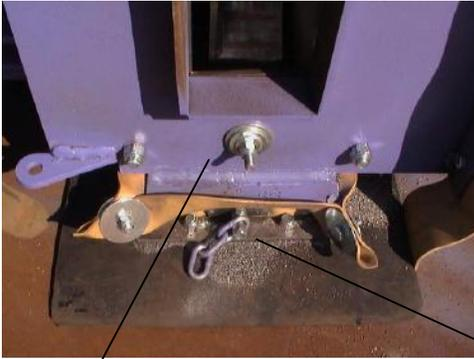
Make sure that the lower liner is in place and bolted securely.
