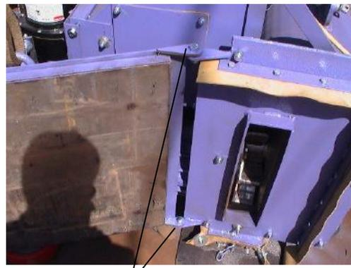
Place the magnet pivot eye mounts on top Of the wall blast plate mounts and attach with (2) 1/2" bolts and lock nuts.
