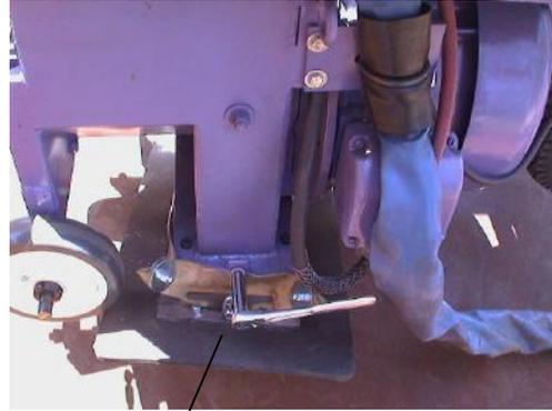
Lift the machine a few inches of the floor, with a fork lift, strap and shackles- see lifting points page . Remove the seal assembly by removing the nut and chain attachments on both sides of the machine.
