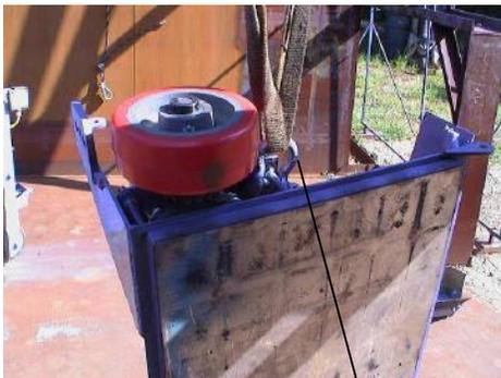
Pick up the magnet/ drive assembly with a fork lift, strap and shackle. Locate the shackle around the threaded rod, as shown, so the unit will hang in a vertical and balanced position.
