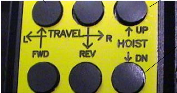
Press and hold down to **Raise** the machine on the wall (vertical mode only). Release to stop.
