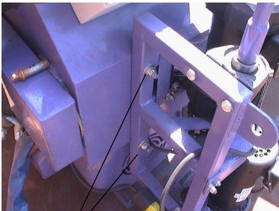
Place the steering assembly on the two studs located on the reclaim hopper. Install washers and lock nuts and tighten.
