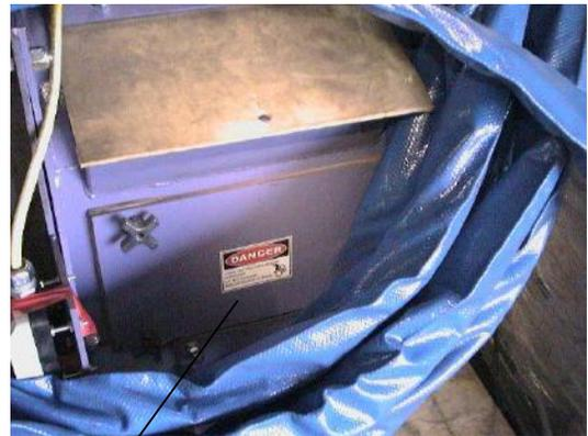
Lock out machine before servicing do not operate without guards in place
