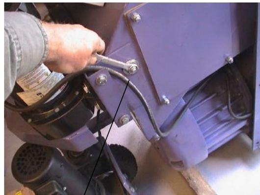
Tighten the lock nut on the side support plate.
