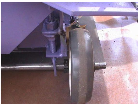
Lift the unit back vertical. Holding the unit slightly off the floor, slide the axle and right tire assembly through the adjustable support.
