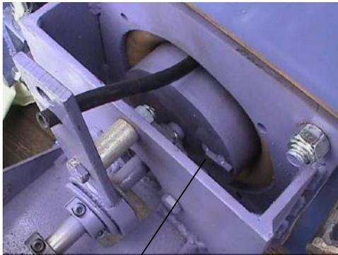
Rotate the arrow on the control cage to 3:00 (as shown) for vertical cleaning.
