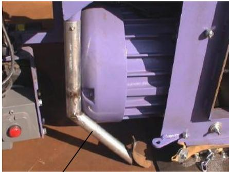
Remove the reclaim drain/ dribble valve
