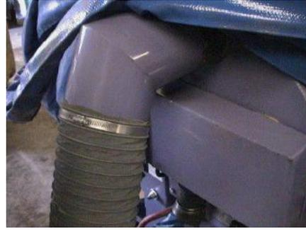
Connect the 6” exhaust hose to the machine and to the dust collector as shown.
