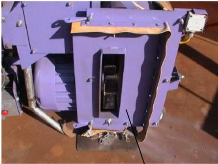
Bolt on the wall blast plate using the (7) 1/2" bolts from the side cover plate.
