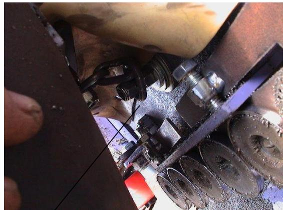
Attach the seal by sliding the chain onto the mounting stud and securing with the lock nut. Follow the same procedure to secure the bottom.
