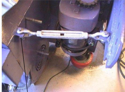
Remove the turnbuckle bolt from the reclaim hopper.
