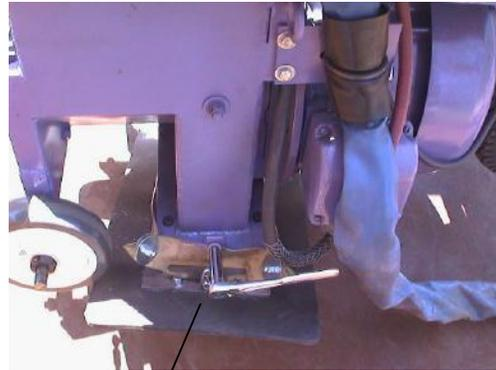
Attach the seal assembly. Slide the attachment chain over the stud and secure with a lock nut. Then secure the attachment chain on the other side of the machine.
