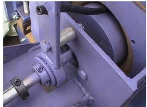
After making the changes slide the locking arm back in place and install the locking bolt, collar and washer.
