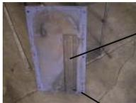
The liner for floor applications is mounted on the side cover plate. Remove the plate and inspect this liner, all blades, the top curved liner, and the back wall liner on 50 hour intervals. If wear is found, remove the liners and fill the wear area with hard face weld. If the wear is too great, replace the liner.
