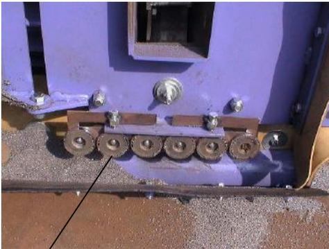
Slide the magnet mount in place as shown. Secure with lock down bolts.
