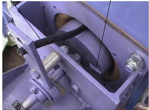
Rotate the control cage clockwise until the arrow on the end of the control cage is at 3:00 to 5:00. Be sure to reinstall the breathing tube.
