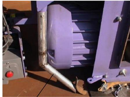
Attach the reclaim drain/ dribble valve
