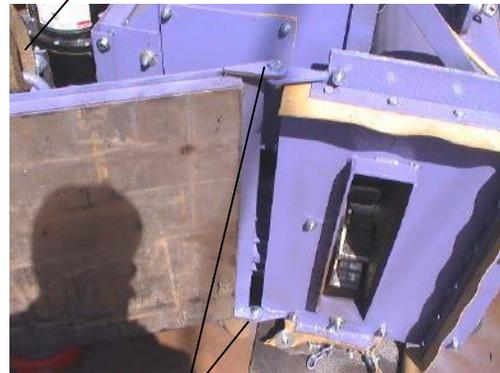
Remove the two 1/2" bolts at the hinge pivot Points and remove the magnet assembly.
