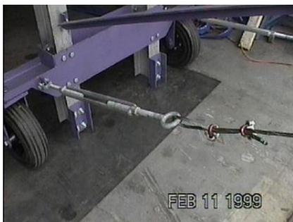
Run the cable from the turnbuckle through the rear eye and around the tanks center stand pipe. Run the cable back through the other rear eye and connect it to the opposite turnbuckle using at least two  $\frac{3}{8}$ " cable clamps. Pull the cable tight as possible before clamping. Next pull the two cables together and place a single clamp about two foot from the stand pipe. This will keep the fixture running square to the tank.
