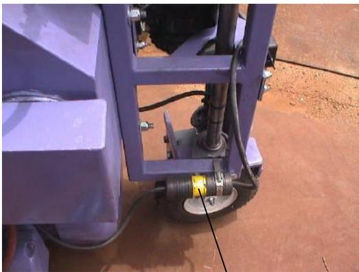
Plug in the steering motor power cord.
