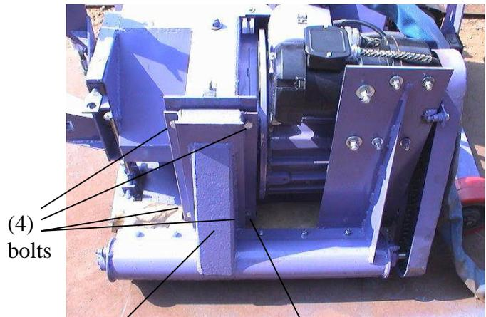
Remove the (4) 1/2" bolts holding the lower reclaim assembly in place. Remove the lower reclaim assembly.
